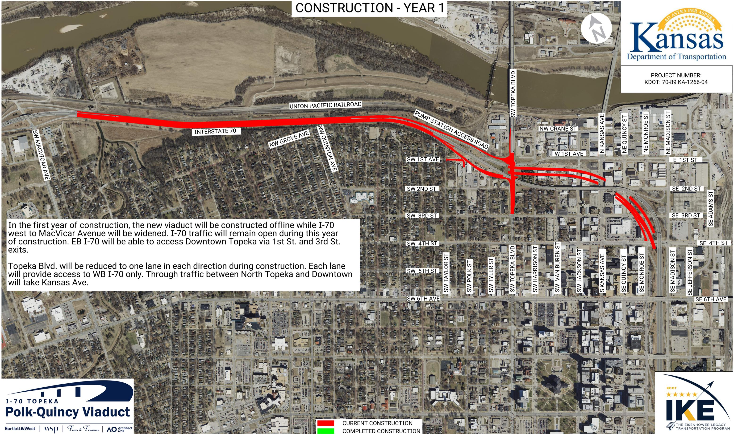
In the first year of construction, the new viaduct will be constructed offline while I-70 west to MacVicar Avenue will be widened. I-70 traffic will remain open during this year of construction. EB I-70 will be able to access Downtown Topeka via 1st St. and 3rd St. exits.
